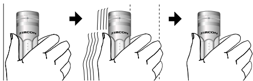
Figure 1: Scanning for AC Voltage
